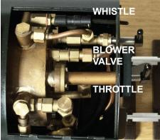
It will take approximately 7 minutes to raise pressure. Once the gauge reaches 20 lbs, you can shut off and remove suction fan from the stack
