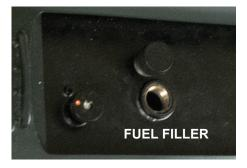
When fueling the locomotive the fuel valve should be shut. Replace filler cap immediately after filling tank. The alcohol will cause the O-ring to dry out, use a small drop of machine oil on the O-ring to keep it pliable.
